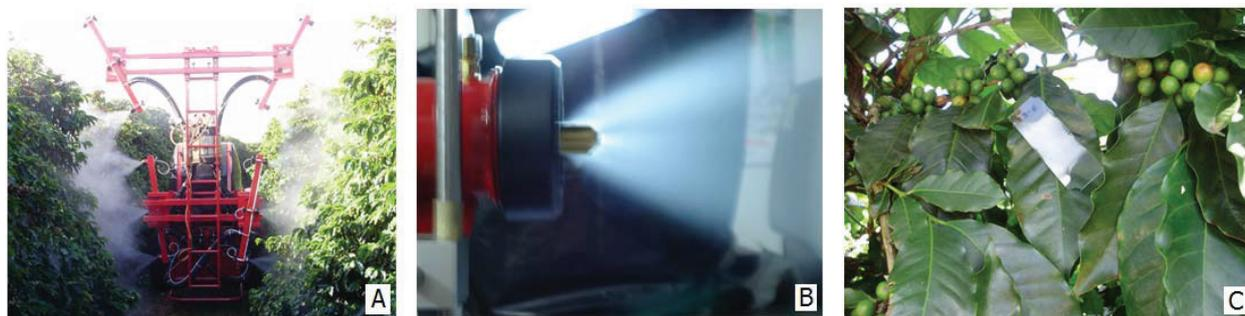
Fig. 1. ULV Sprayer (A), pneumatic flat spray nozzle (B) and the glass slide coated with magnesium oxide (C).
