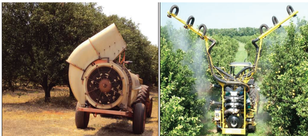
Fig. 1. Models of sprayers used in experiments to evaluate the control of Citrus Black Spot and juice quality. Arbus 2000 (Conventional) on the left and TOPSpray (surrounding sprayer) on the right.
